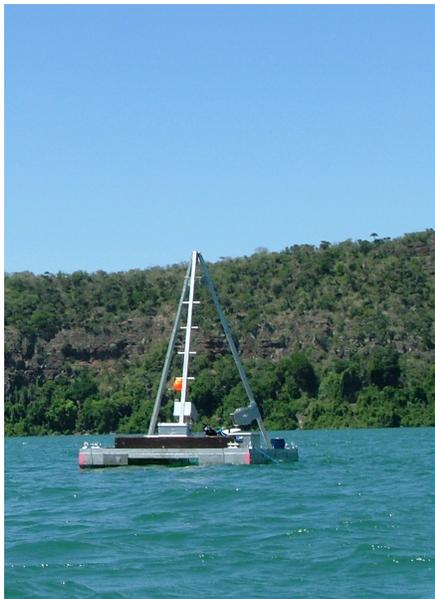
Figure 1. Sediment Drilling Platform. Photo courtesy Stephan Opitz.
