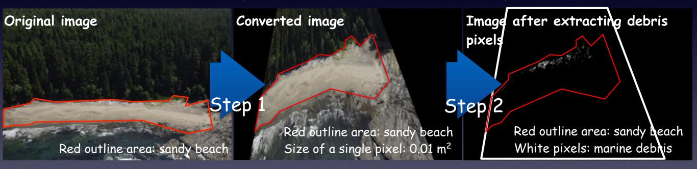
Step 1: Removing the distortion of the original image (Magome et al., 2007)
