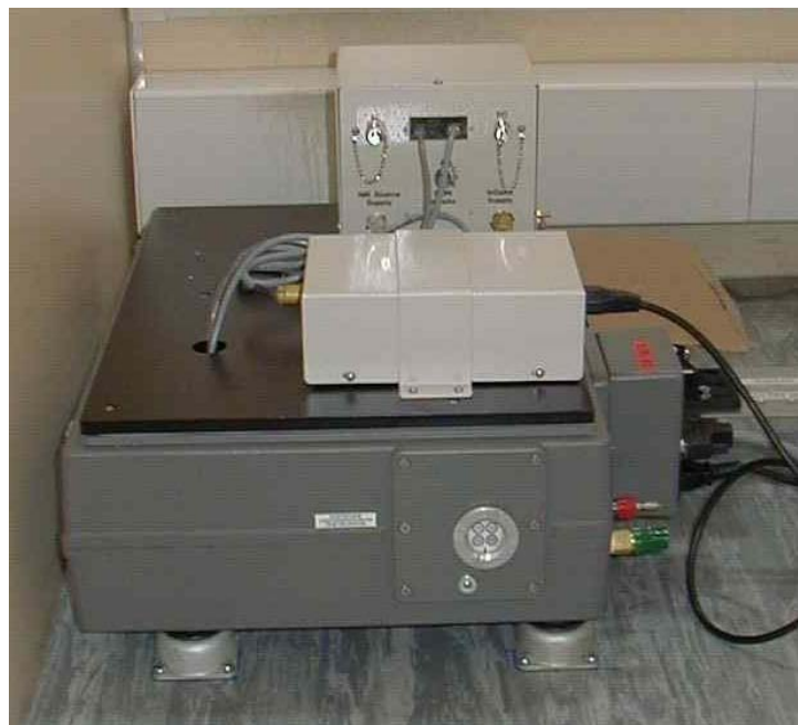
Michelson Interferometer 4 \text{cm}^{-1} Resolution
