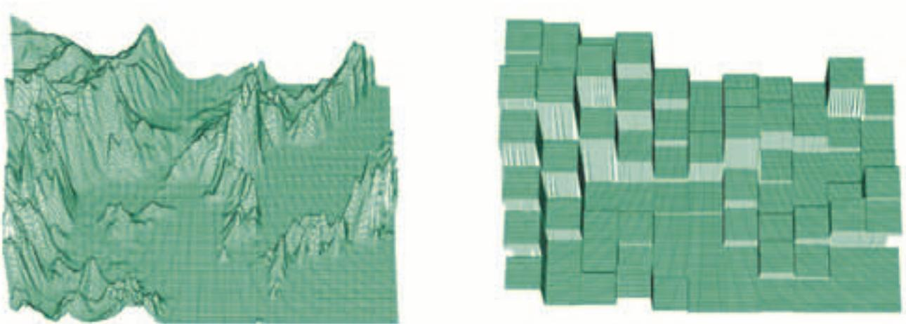
**Figure 8.** A northward-looking view of the topography of parts of East Asia: Southeast Asia is in the lower left corner, Korea near the center, and Japan on the right. Left panel: The topography in the T1279 version of the AFES model. Right panel: the mean values for grid squares with dimensions of about 300x300 km, the typical resolution in a present-day model applied to long climate integrations.
