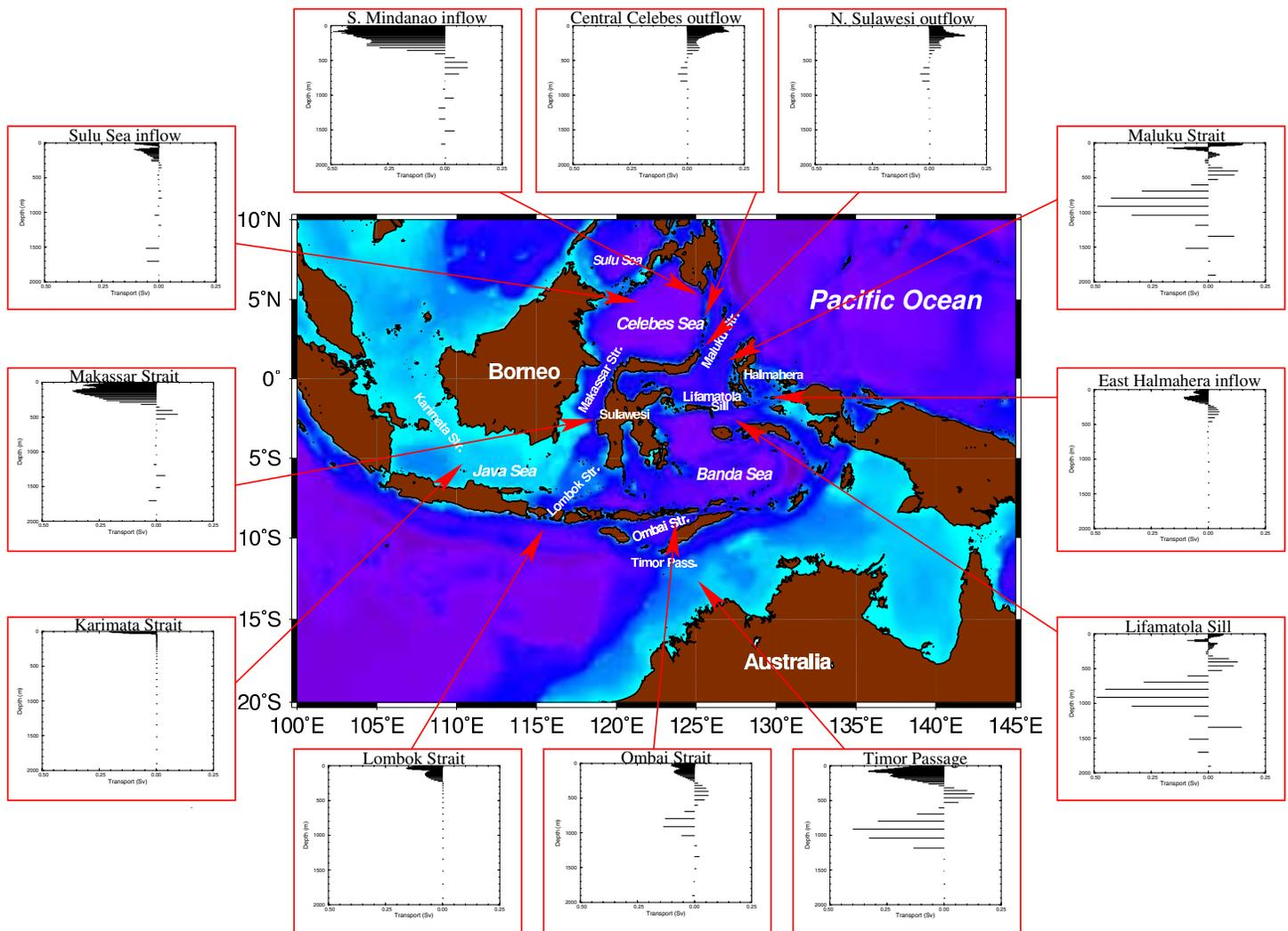
**Figure 10.** A map of the main straits in the Indonesian seas together with bathymetry (5,000; 1,000; and 100-m depths are shaded). Depth-integrated transport from the OFES, as a function of depth, is given for selected straits. Negative values indicate southward or westward flow.
