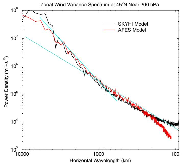
**Figure 9.** The zonal wavenumber spectrum of the variance of the zonal wind along the 45°N latitude circle at 200 hPa. Results for simulation with the GFDL SKYHI model (black) and for the AFES (red). The straight lines are drawn for reference and show  $-3$  and  $-5/3$  power-law slopes.
