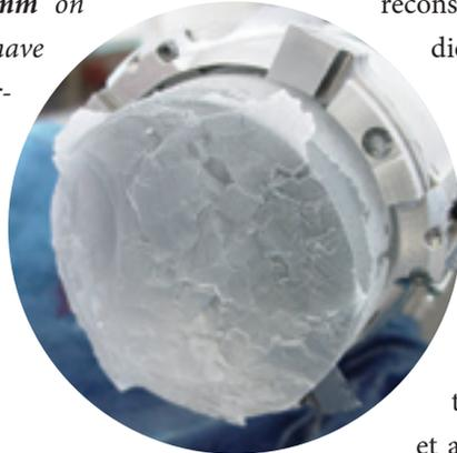
**Above.** Drill head with ice core drilled on November 30, 2002, from a depth of 2,874 m at Dome Concordia Station. The ice is about 491,000 years old. The drilling is part of the European Project for Ice Coring in Antarctica (EPICA). This ice core contains a continuous time series of greenhouse gases over the last 650,000 years. The drill head and cutters were designed and constructed by Henry Rufli (University of Bern, Switzerland; photo courtesy of L. Augustin, LGGE, Grenoble, France).
