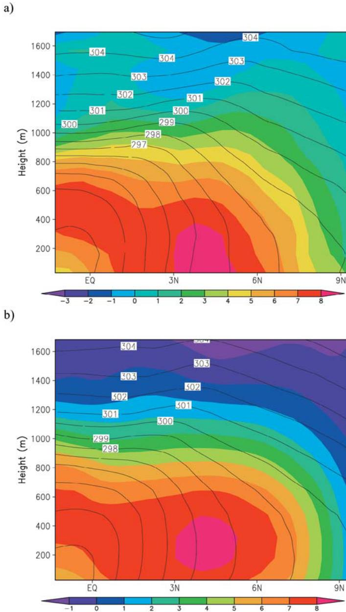
**Figure 3.** Vertical sections of meridional velocity (color, m/s) and potential temperature (contours: intervals of  $1^{\circ}\text{K}$ ) at  $95^{\circ}\text{W}$ : (a) from EPIC2001 NCAR C130 data (8-flight mean); and (b) from the IPRC-RegCM (2-month mean).
