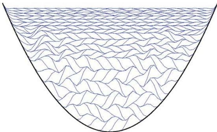
**Figure 1:** The initial distribution of sacks in a parabolic lake. Placing small sacks at, and near, the surface resolves the temperature stratification near the surface. In the deeper part of the lake, temperature is more uniform, so that larger sacks may be used to save computing time.
