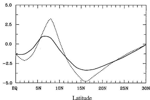
FIG. 7. The time tendency for SST (units:  $10^{-8} \text{ K s}^{-1}$ ) at  $t = 0$  in the cases of linear (solid line) and nonlinear (dotted line) atmospheric heating, in the presence of the evaporation–wind feedback.
