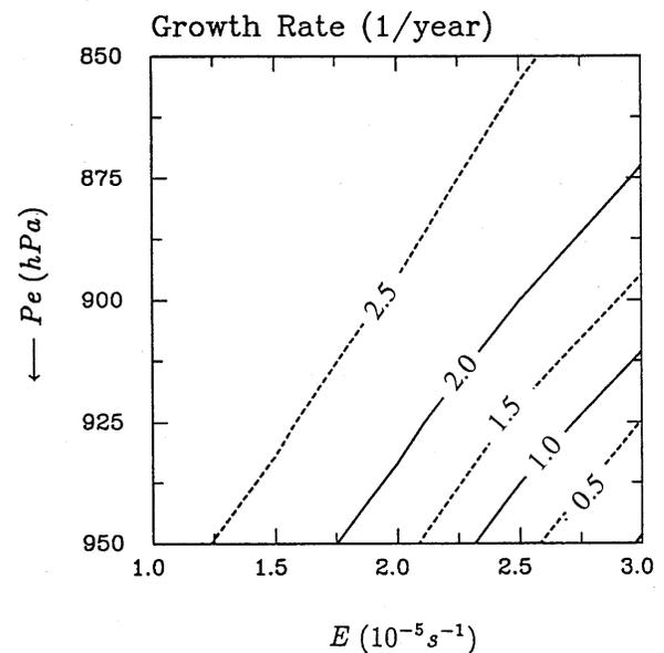
FIG. 5. Growth rates ( $\text{yr}^{-1}$ ) as a function of (a) the basic-state vertical temperature gradient and friction coefficient in the ocean mixed layer and (b) the pressure at the top of the atmospheric boundary layer and the Ekman number in the presence of the meridional wind–SST feedback.
